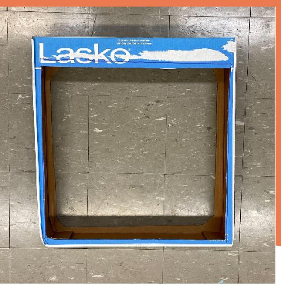
On the other side, cut a square with rounded corners that is 1/2inch smaller all around compared to the fan's size.
