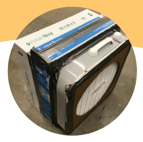
Tape the shroud to the other side of the fan that is not attached to the plenum.
