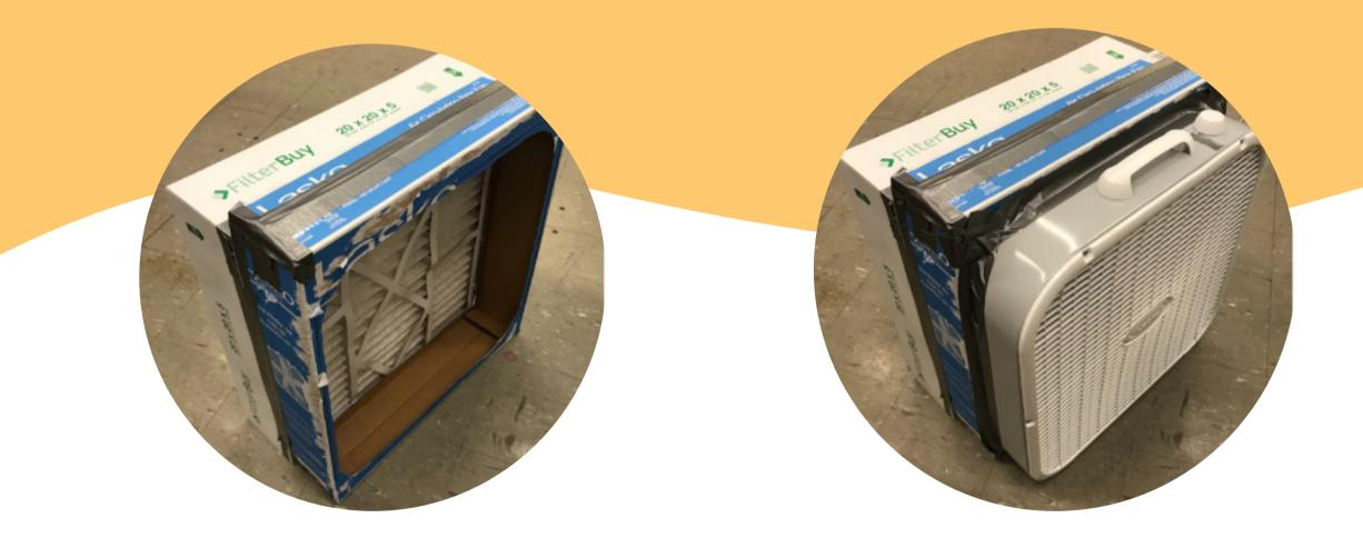
Tape the air filter (with the arrow on top of the filter facing toward the plenum) to the side of the plenum that matches the filter's face dimension Tape the back of the fan to the free side of the plenum
