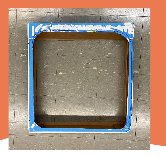
Get the cardboard box where the fan came in and on one side, cut a square that is a 1/2 inch smaller than the air filter size.
